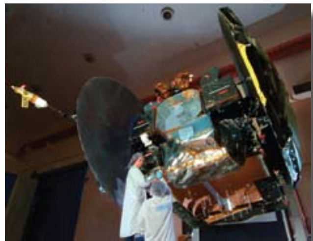
Built on the Space Systems/Loral 1300 satellite bus, MTSAT-1R has two payloads, one that provides aeronautical services and one for weather monitoring.
