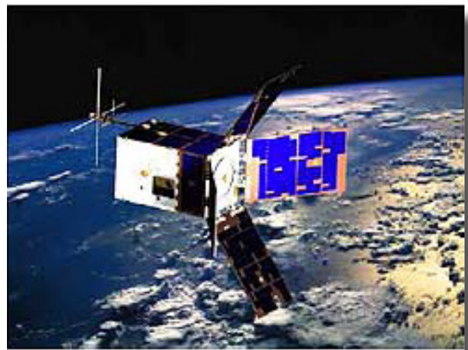
Illustration of fully-deployed STPSat-1 SV on orbit, with CITRIS antenna on SV front, and circular standard separation adapter on back.
