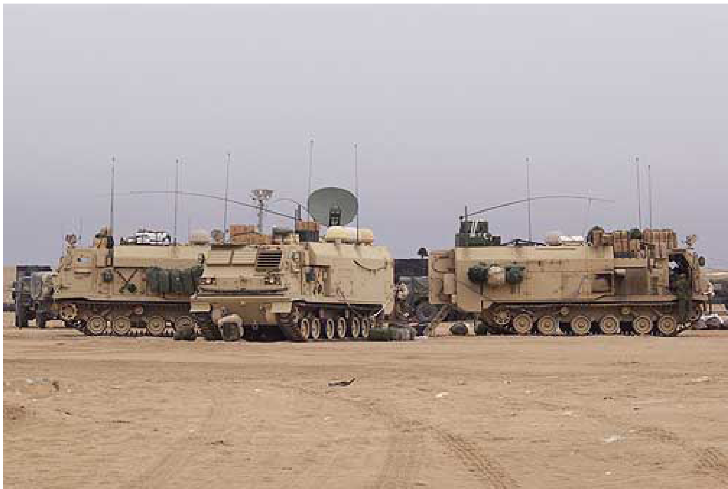
U.S. V Corps' Assault Command post, Western Iraq, 2003. A SWE-DISH DA150K satellite antenna mounted on top of LTG Wallace's Command and Control Vehicle. Satellite communications enabled him, as the first US commander in modern history, to lead his troops from the front.
