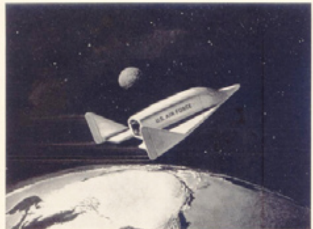
SPACE GLIDER. Drawing of Dyna-Soar space glider, which will maintain extreme speed of a ballistic missile with controlled and accurate flight of a manned aircraft. Designed to fly in orbit in low space, where it could travel at speeds approaching 10,000 mph. Dyna-Soar will be able to re-enter earth's atmosphere and make conventional pilot-controlled landing. Boeing is prime contractor for Dyna-Soar, now being developed by U. S. Air Force with cooperation of National Aeronautics and Space Administration.
