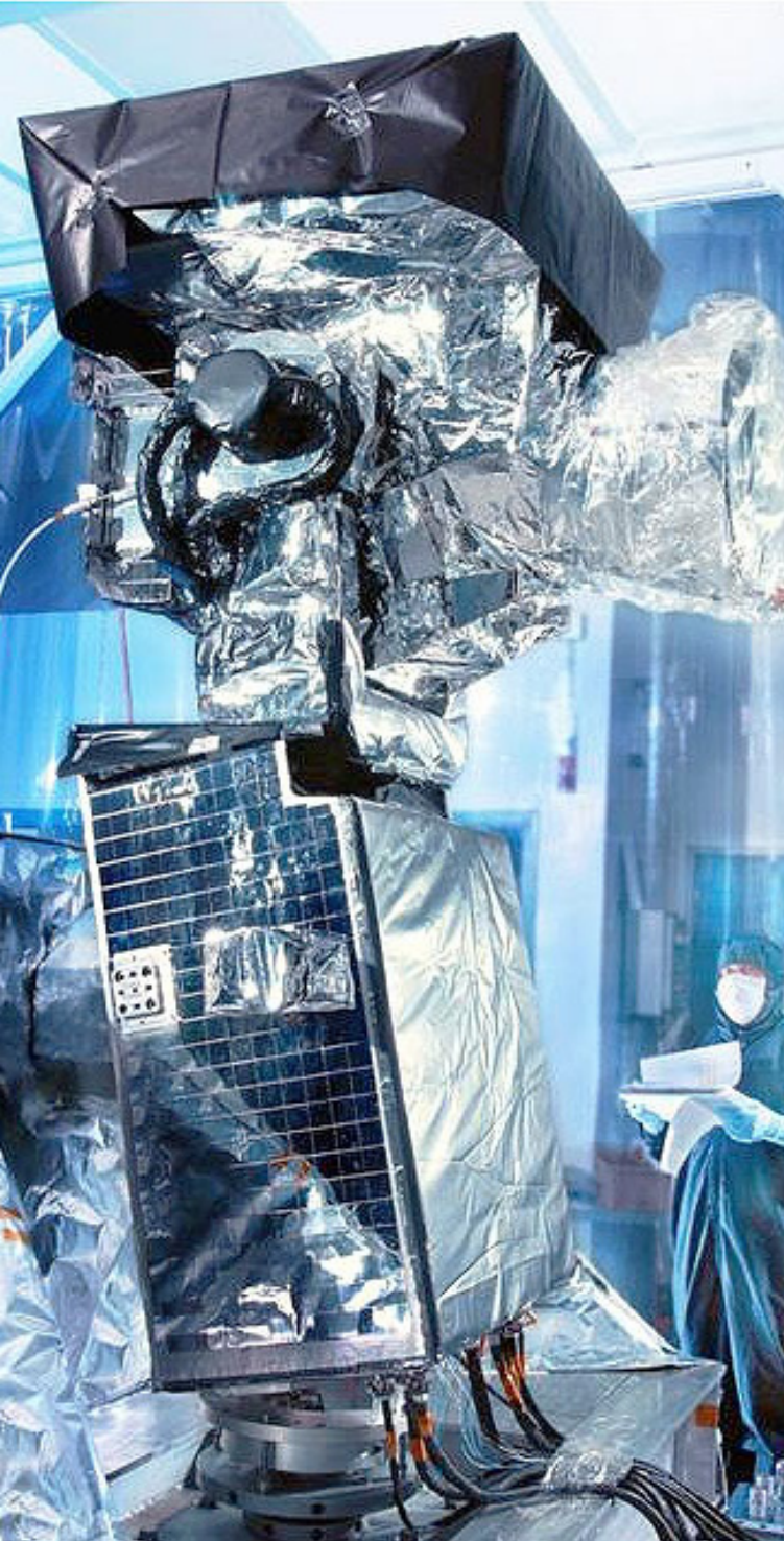
Lockheed Martin's thermal vacuum testing of the Space Based Infrared System (SBIRS) geosynchronous (GEO-1) satellite, photo courtesy of Lockheed Martin
