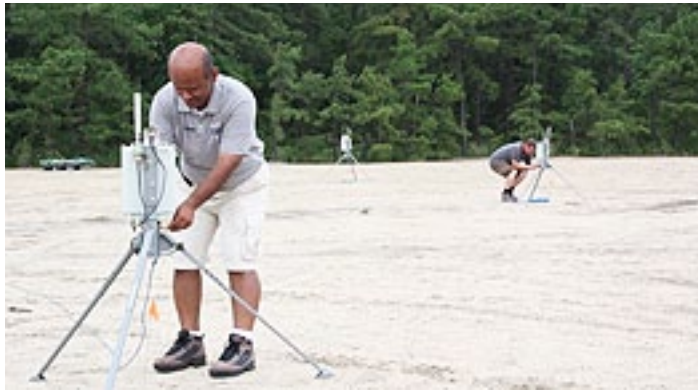
(Left to right) Mitesh Patel, technical lead for the Cognitive Algorithm & Network Design Experiment, and Eric Williams of C4ISR & Network Modernization inspect radios during an E11 test. The CANDE algorithm can determine which tactical radio signal has the best bandwidth or least traffic before transmitting data.
