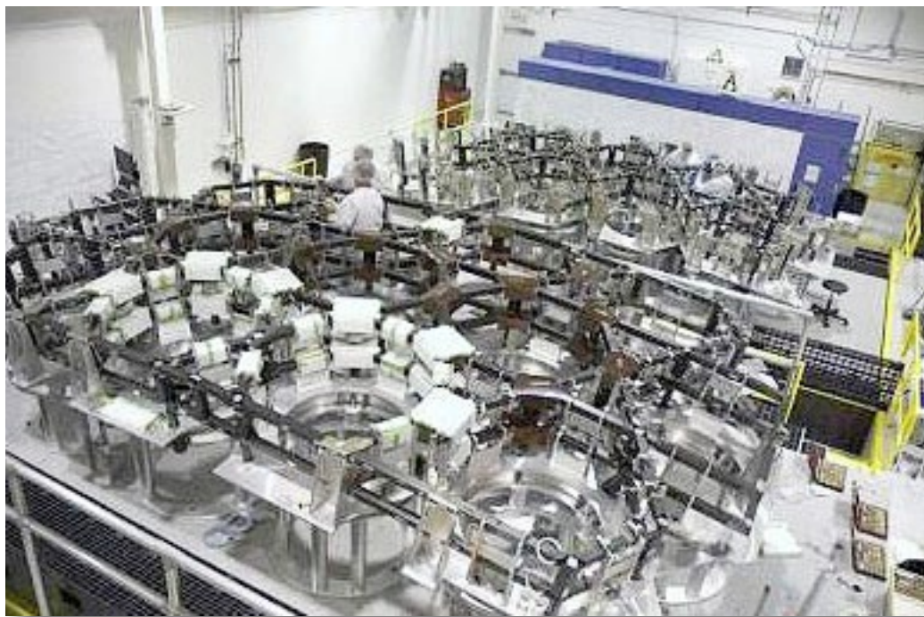
The James Webb Space Telescope pathfinder backplane during the manufacturing process
