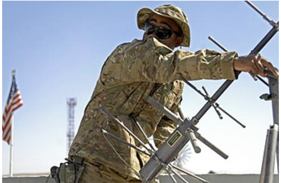
Staff Sgt. Joel Crowder, Provincial Reconstruction Team Zabul communications non-commissioned officer in charge, adjusts a Satellite Communication Antenna, Forward Operating Base Smart, Afghanistan, Oct. 18, 2011. PRT Zabul's Communications experts adjust and maintain equipment to ensure that the team remains connected to the rest of the battle space.
