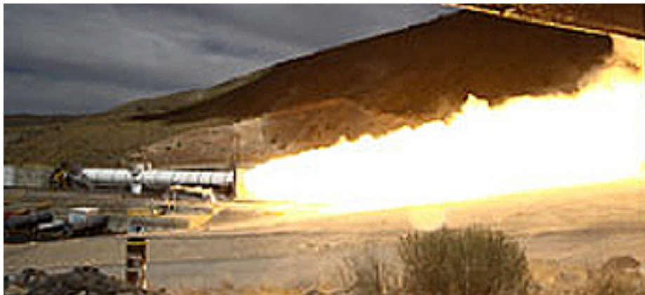
ATK and NASA's successful ground test of the second, five-segment, solid rocket motor, furthering the design of a new rocket motor for use in America's future heavy lift launch vehicles.
