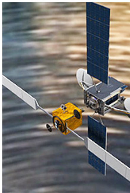
The MEV about to dock with a satellite for refueling purposes.
