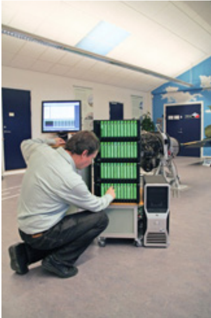
High channel counts and high sampling frequencies necessitate advanced data acquisition systems. Here an engineer sets up Brüel & Kjær's modular LAN-XI platform.
