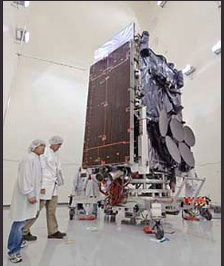
Technicians surround a Wideband Global SATCOM in the acoustic chamber at the Boeing satellite manufacturing facility in El Segundo, California. WGS satellites will serve as USAF's communications workhorses for some time forward. (Photo courtesy of Boeing)
