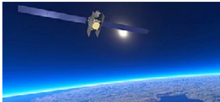
HUGHES' SPACEWAY® 3 satellite is a high-capacity commercial satellite and offers onboard switching and routing.
