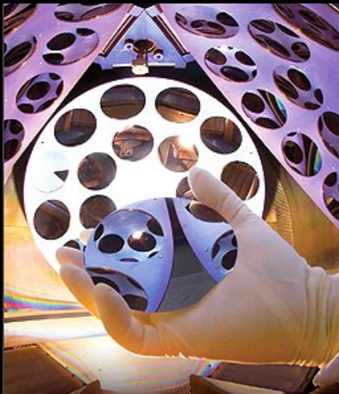
A technician holds a germanium wafer at Spectrolab. Ultra-triple-junction gallium arsenide solar cells are grown onto the wafers using specialized machine]
