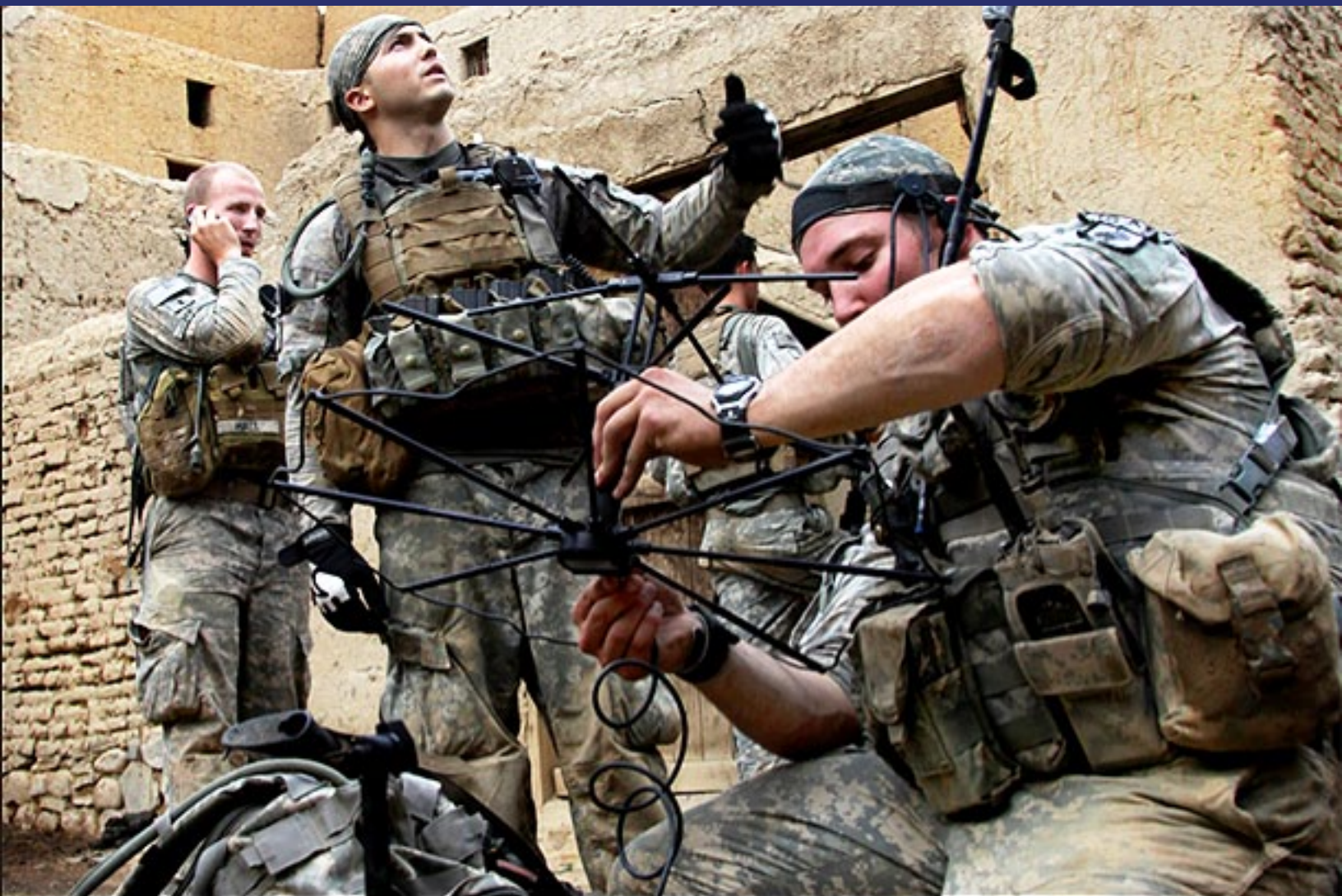
U.S. Soldiers with 2nd Platoon, Attack Company, 1st Regiment, 503rd Infantry Battalion, 173rd Airborne Brigade Combat Team set up a tactical satellite communication system in Shekhabad Valley, Wardak province, Afghanistan. Photo by Sgt. Russell Gilchrest
