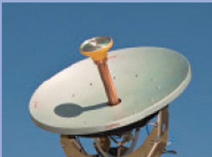
Tachyon's 18-inch Ku-band antenna, used for the MARSS program.
