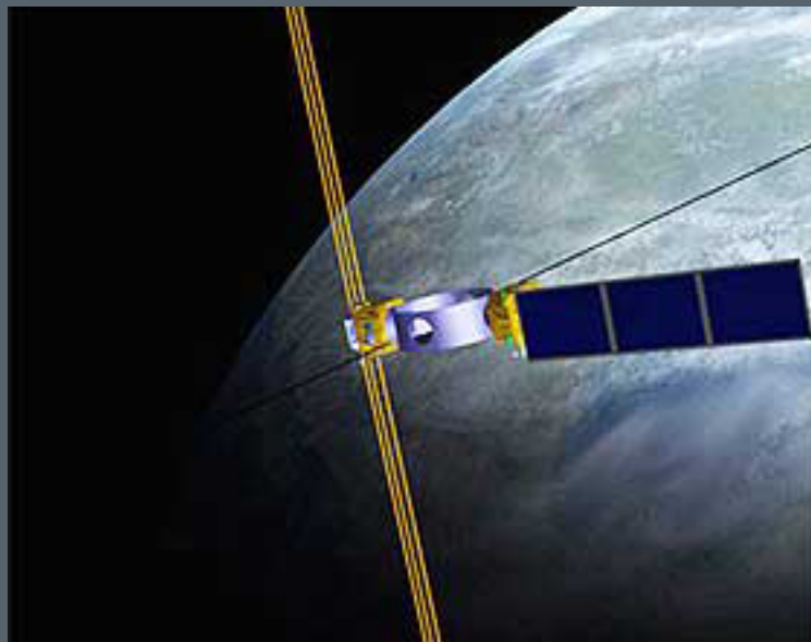
Artistic rendition of the U.S.A.F.'s DSX, which includes four science payloads that will be integrated onto an ESPA ring.
