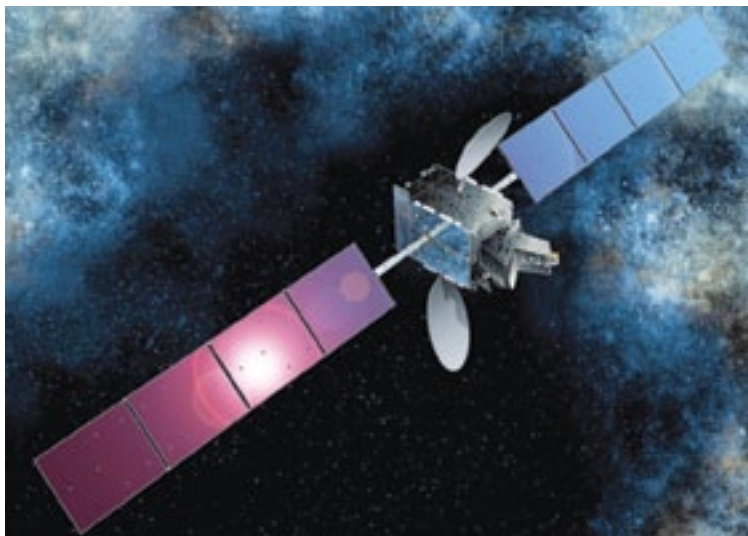
The SES-5 satellite, also known as Sirius 5, includes an L-band hosted payload for the EU... the payload is part of EGNOS, which is being developed by the ESA and the EC. The successful launch occurred on July 10, 2012, via an ILS Proton-M launch vehicle.
