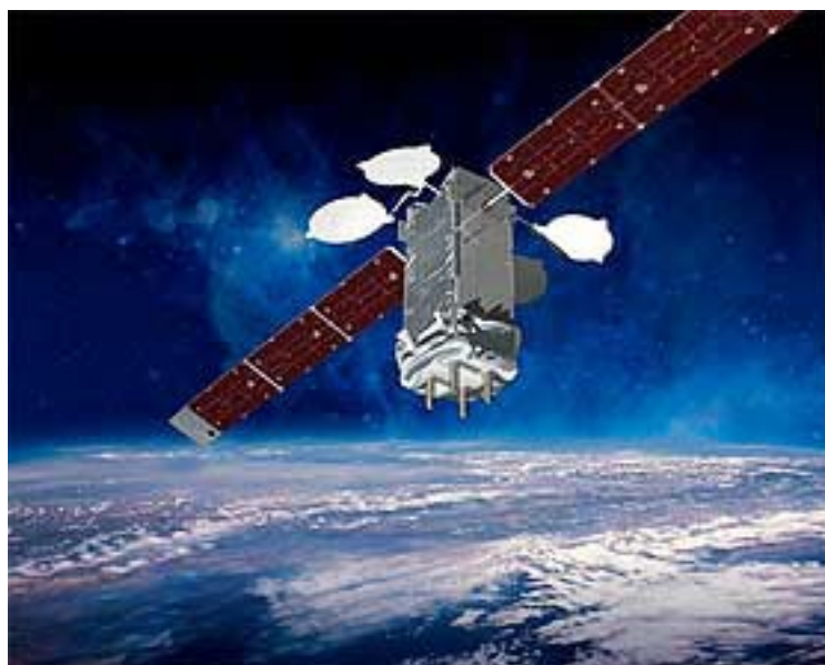
An artist's rendering of a Boeing satellite with a hosted payload. The hosted payload is the four-pronged square facing toward Earth. Image is courtesy of Boeing.
