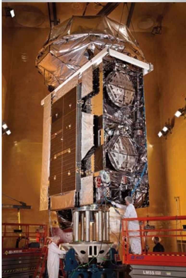
Lockheed Martin engineers prepare the third Mobile User Objective System (MUOS) satellite for acoustic testing, one of several simulated environmental tests to validate the satellite's performance throughout its launch and on orbit mission life. Photo courtesy of Lockheed Martin.
