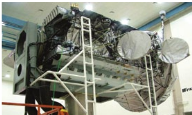
Figure 5. The first MUOS satellite completing thermal/vacuum testing at the Lockheed Martin facility in Sunnyvale, California.
