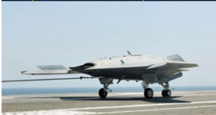
Northrop Grumman and the U.S. Navy complete the first arrested landing of a Tailless Unmanned Aircraft aboard an aircraft carrier.
