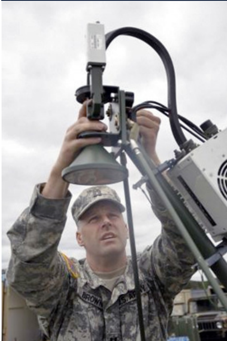
U.S. Army Capt. Frank Brown, communication officer with Headquarters and Headquarters Detachment, 213th Regional Support Group, Pennsylvania Army National Guard, attaches a feed horn to the stabilizing arm of a portable satellite system during exercise Golden Coyote at Forward Operating Base Custer at Custer State Park in Rapid City, South Dakota, June 5, 2013. Golden Coyote is an annual training exercise that joins U.S. Service members from 11 states and Soldiers from four foreign nations.
