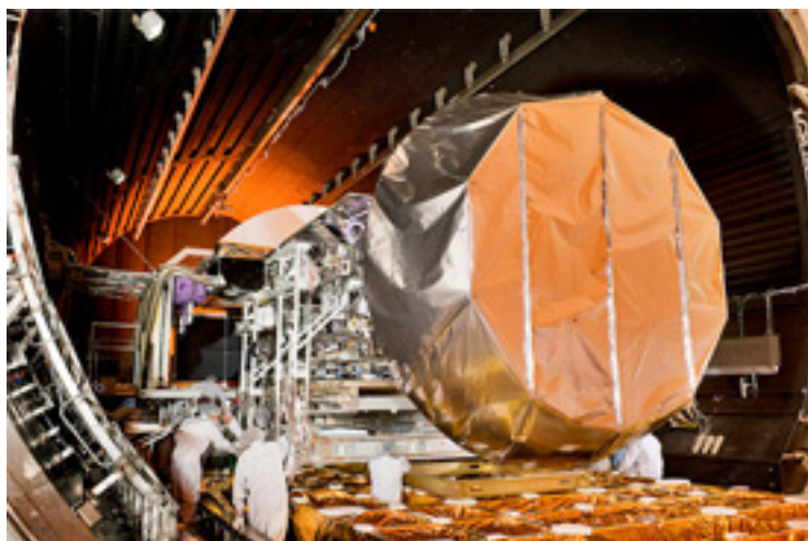
MUOS-2 undergoing environmental testing. Photo courtesy of Lockheed Martin.
