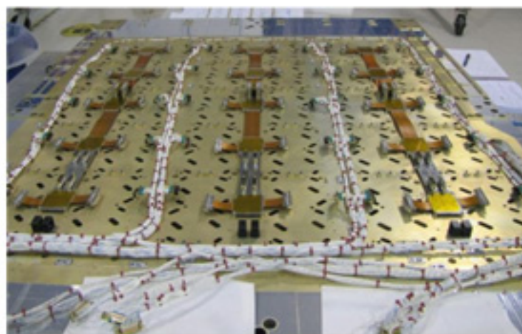
The ATK Equipped Structural Panels provides Mechanical Structural Support, Thermal Control, and Electrical Functional Harnessing for the Iridium Next Main Mission Antenna
