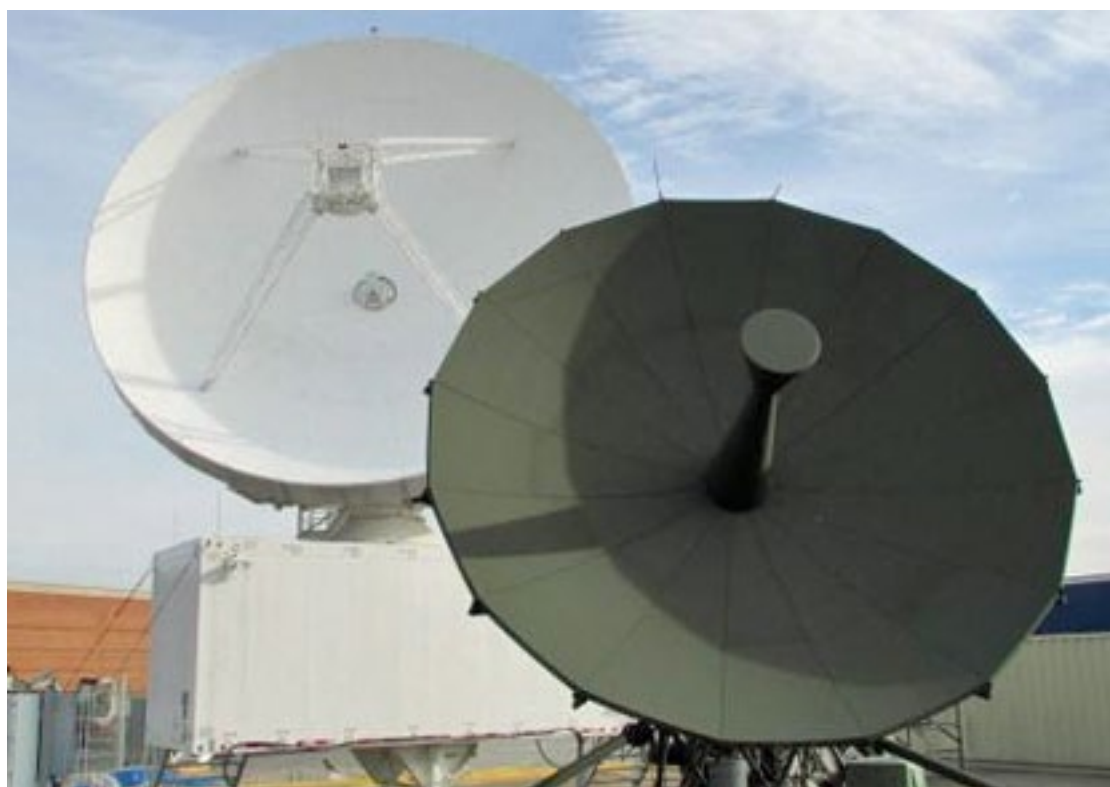
Two terminal dishes assist Army space soldiers of Alpha Company, 53rd Signal Battalion (SATCON) at the Wideband Satellite Communications Operations Center, Fort Detrick, Md. The green antenna is called a replacement terminal and is temporarily supporting A Company's Auxiliary Site Control Terminal mission, while the Modernized Enterprise Terminal (white antenna) is going through testing in preparation to fill a Wideband Global Satellite and ASCT role. The MET is the latest antenna to be fielded with several upgraded capabilities. This facility provides Alpha Company controllers increased capabilities to control the communications payloads and communications transmissions of the Defense Satellite Communication System and WGS constellations.
