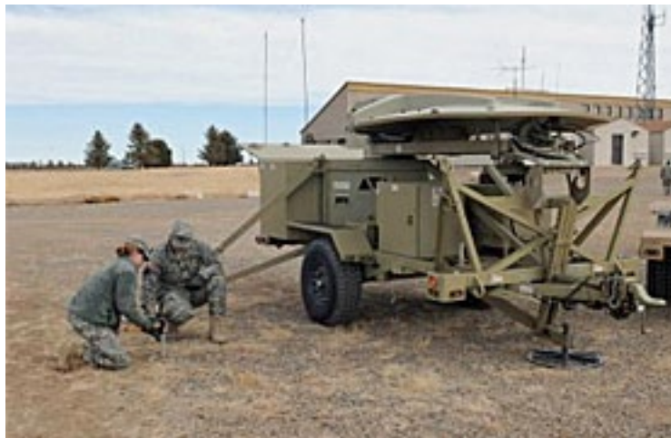
U.S. Army Sgt. Danielle Dye, left, and Spc. Reynold Studler, place grounding stakes for a satellite terminal at Pinon Canyon Maneuver Site during training in Trinidad, Colo., Feb. 19, 2013. The satellite terminal allows units to have connectivity and to send and receive data in a field environment. Dye, a multichannel transmission systems operator maintainer and Studler, a cable system installer are both assigned to Bravo Company, 2nd Special Troops Battalion, 2nd Brigade Combat Team, 4th Infantry Division. (U.S. Army photo by Staff Sgt. Andrew Porch/Released)
