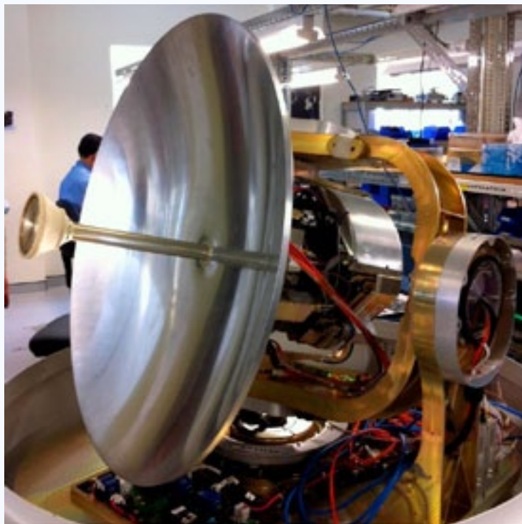
Figure 3. The parabolic reflector and Ka-band antenna feed system, which rotates to match the polarisation of the incoming signal
