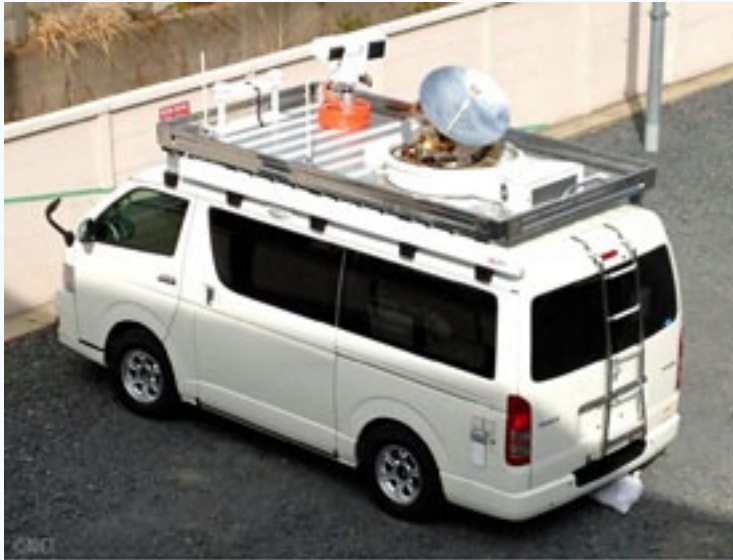
Figure 1. EM Solutions broadband on-the-move terminal being readied for operation atop a communications node being deployed for disaster recovery operations.
