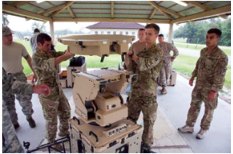
Two members from the UK's 30th Signal Regiment, U.K. Cpl. Tommy Bamford (center left) and a fellow team member, build familiarity on the Joint Communications Support Element's (JCSE) Hawkeye 2.4m multiband satellite terminal.
