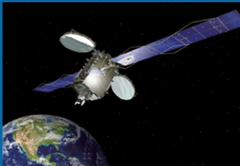
The Commercially Hosted Infrared Payload (CHIRP), a heat-detecting sensor installed on the SES-2 communications satellite—this mission demonstrated that commercial satellites can host military or intelligence sensor payloads without interference. Image is courtesy of Orbital Sciences Corp.
