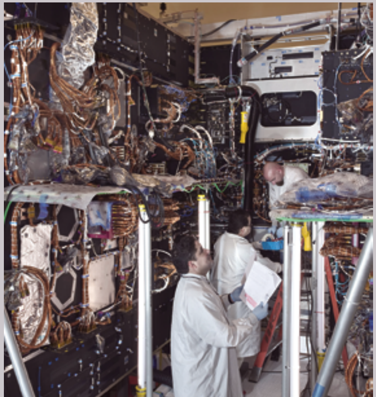
Another photo of the Advanced EHF protected communications payload during integration and testing at Northrop Grumman in Redondo Beach, California. Photo courtesy of Northrop Grumman.
