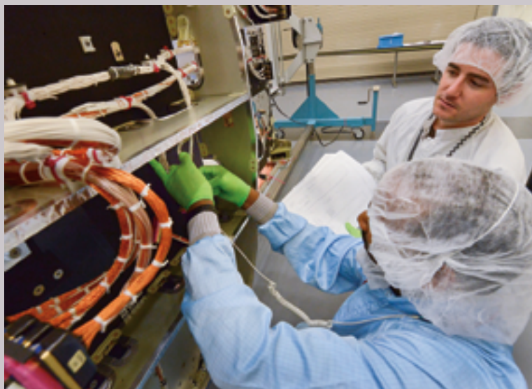
Northrop Grumman technicians thread wiring and cabling through the fourth protected communications payload for the U.S. Air Force's Advanced Extremely High Frequency satellite system. (Northrop Grumman photo.)
