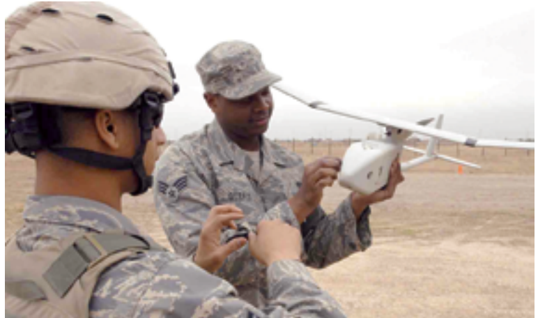
The GPS MUE GPS receiver module is intended for platforms such as the Raven uncrewed aerial vehicle, shown here in preparation for launch. U.S. Air Force photo/Senior Master Sgt. Don Senger
