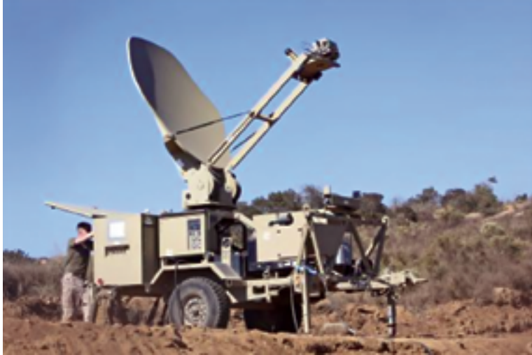
Sergeant Christopher Phillips, a satellite communications operator with Communications Company, Combat Logistics Regiment 17, 1st Marine Logistics Group, operates a satellite terminal during a CLR-17 combat operations exercise aboard Camp Pendleton, California. Approximately 100 Marines with Communications Co. worked on setting up data, radio and wire communications systems at three sites to enable CLR-17's logistical elements to function and support other forward units with the 1st MLG. (U.S. Marine Corps photo by Lance Cpl. Shaltiel Dominguez/ Released)
