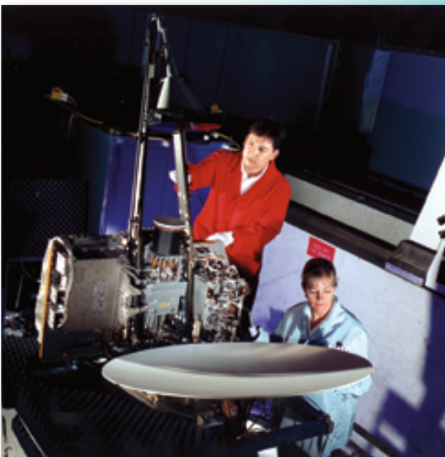
Technicians adjust a nulling antenna for a Milstar protected communications payload. Photo is courtesy of Northrop Grumman.
