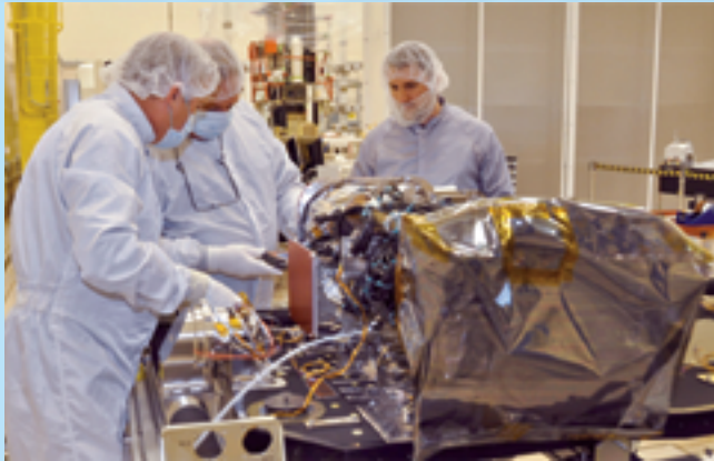
Lockheed Martin engineers in Denver install the Solar Ultraviolet Imager (SUVI) on the GOES-R Sun Pointing Platform. SUVI was built at the Lockheed Martin Advanced Technology Center in Palo Alto, California. Photo is courtesy of Lockheed Martin.
