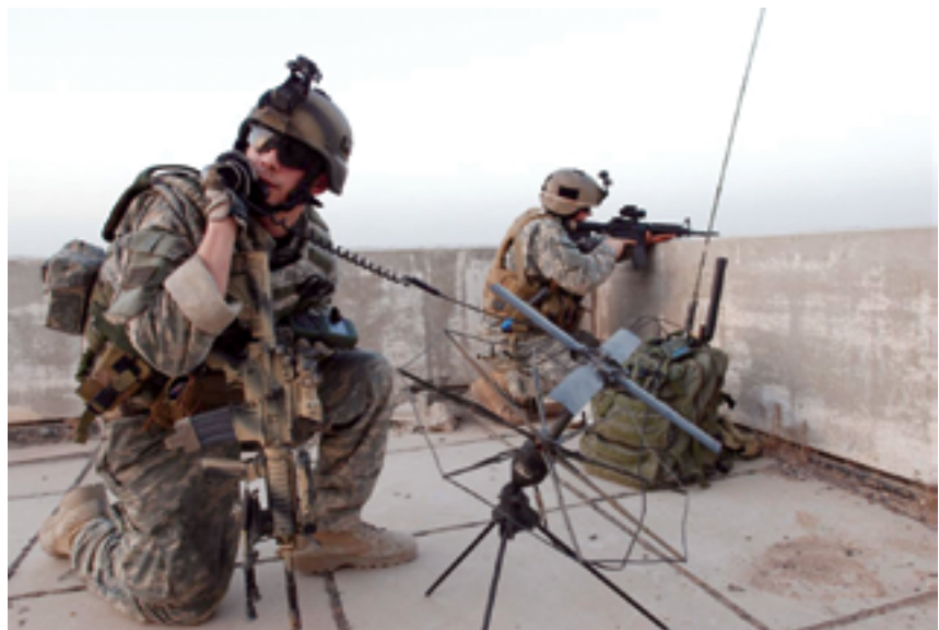
Tactical Air Control Party specialists provide over-watch of friendly forces in an undisclosed location using a PSN-13 global positioning system and an AN/PRC-117F multiband manpack radio. TACPs use a variety of equipment to call in close-air support for ground forces. The TACP-Modernization program office at Hanscom AFB, Massachusetts, is charged with equipping TACP Airmen with the necessary communication tools.
