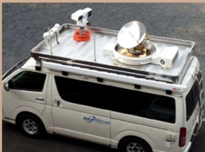
Figure 2. OTM terminal fitted to Vehicle in Japan
