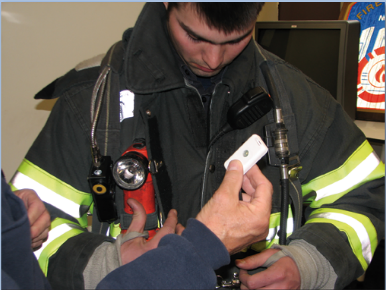
Fire Department New York uses a U.S. Naval Research Laboratory (NRL) system to automatically track firefighters. "That's the intention with this device, to make sure everyone's accounted for," says David DeRieux, one of the inventors. The NRL worked with firefighters to determine where to add the RFID pocket.
