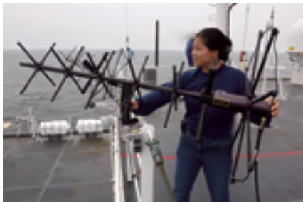
Amy Sun, an advanced program lead for Lockheed-Martin, adjusts a UHF antenna aboard the Coast Guard Cutter Healy while underway near Alaska. Sun works with narrowband military satellite systems and is aboard the Healy to test the capabilities of the Mobile User Objective System in the Arctic. USCG photo by Petty Officer 1st Class Shawn Eggert.
