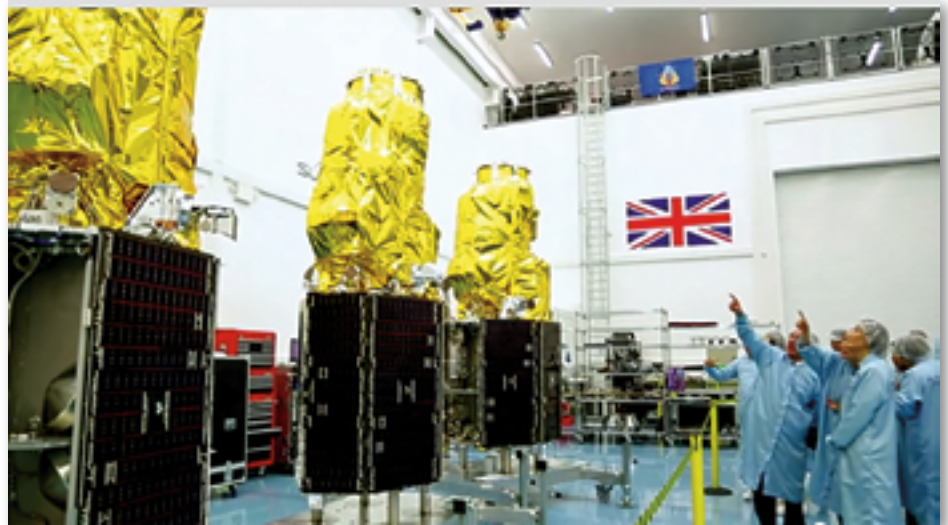
The final assembly and build phase of the DMC3 Constellation satellites at SSTL's cleanrooms in Guildford UK. Photo is courtesy of SSTL.
